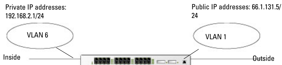
Figure 4 Example: Source NAT using Controller IP Address
